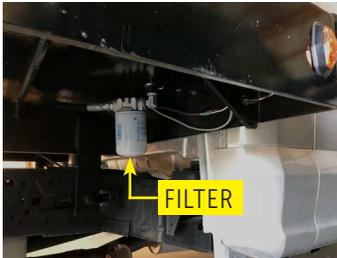
**1** Turn truck and system OFF. Place container under oil filter to catch oil.
